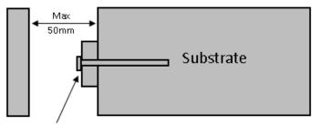
Fix with a 6mm diameter large flanged washer 4 per 1200mm
