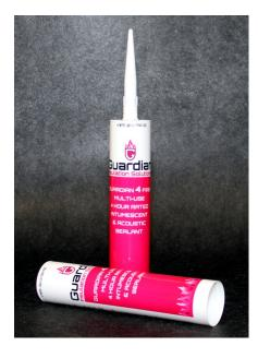
Guardian 4 Fire acrylic is a halogen free, polymer emulsion based sealant that swells when subjected to temperatures in excess of 125oC and forms a char coat that restricts the passage of smoke and fire. It is easily applied and dries to a flexible and smooth surfaced material which is readily over paintable. It has excellent adhesion to a wide range of substrates and will not harden or crack with age.
